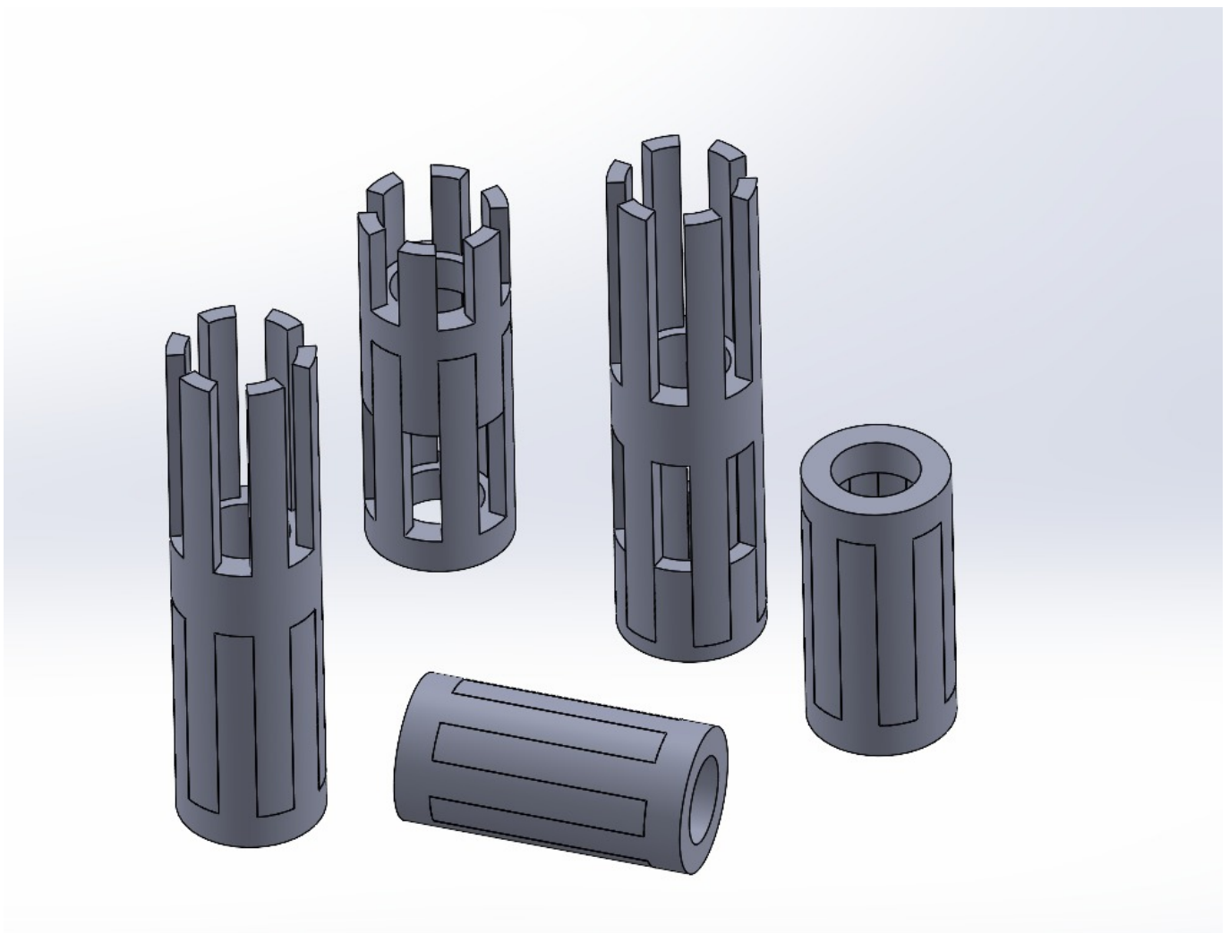
Figure 40: Structural variation exploring different opening sizes and configurations.
