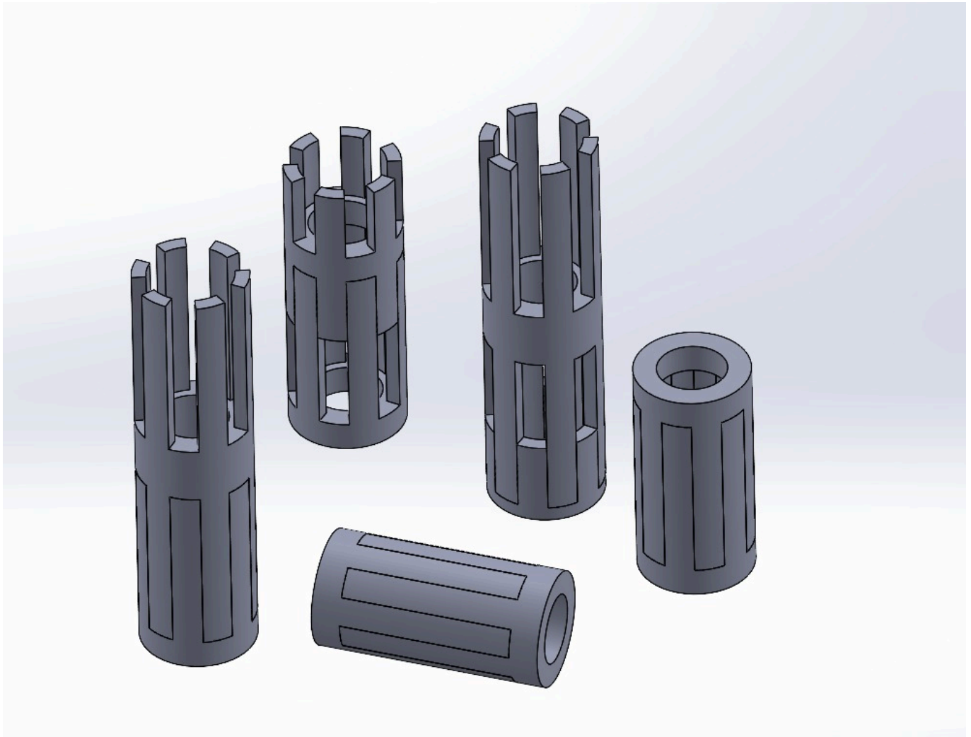
Figure 26: Structural variation exploring different opening sizes and configurations.
